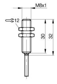
**Inductive Sensors** BES 516-300-S292-BO-D-PU-05 M8x1 x 34 normally-closed **Sn=1,5mm** shielded pressure rated to 100 bar
